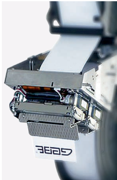
The GeBE-COMPACT, designed as a double printer, processes different paper stock.
